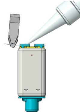
7. Keep soldering iron tip in contact with wire and terminal until solder on wire and solder on terminal pad liquefy and flow into each other. Remove soldering iron tip immediately and hold wire in place with tweezers until solder solidifies. Total time soldering iron tip is in contact with the wire and terminal should not exceed 3 seconds if tip temperature is correct and wire pre-tinning is adequate.
