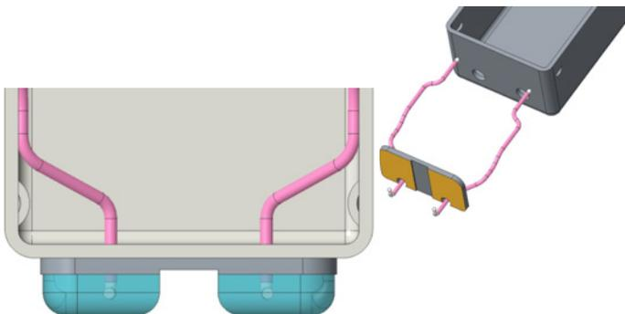
For some microphone families, the internal circuit hybrid extends to the outside of the case as shown in Figure 3. The terminals are located on this section of the hybrid board and are typically “tinned” with SAC305 lead-free solder.
