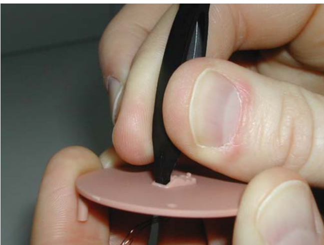
Simultaneously rotate tool away from pushbutton while gently applying force upward
