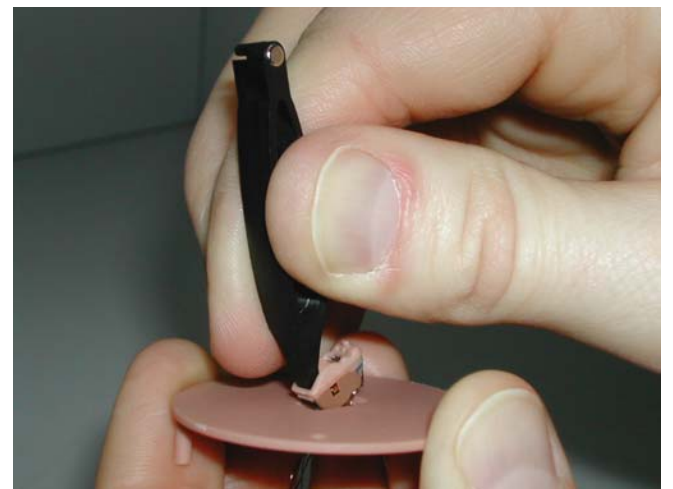
Module detaches from faceplate as shown.
