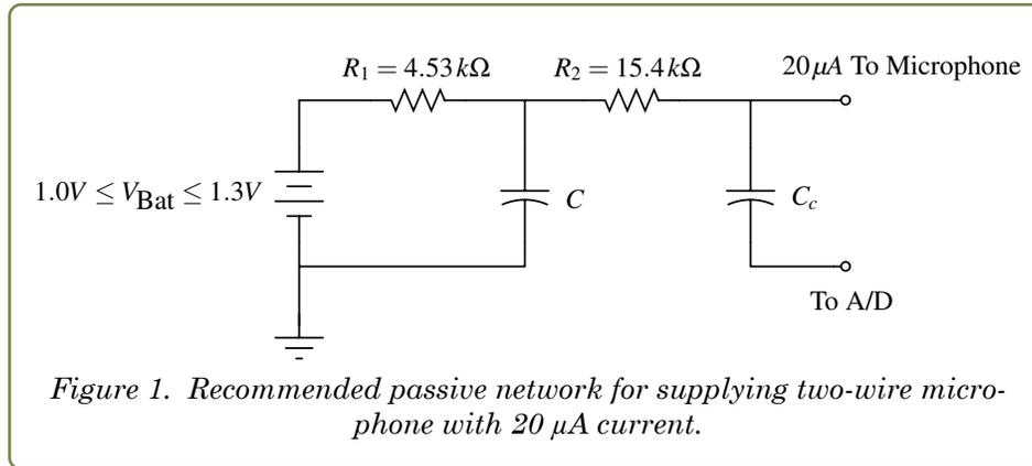
Many Knowles microphones require three terminal connections, one each for supply voltage and ground, and a third for the output signal from the microphone. A Knowles two-wire microphone has only two terminal connections, where the supply and signal are on the same pin. The microphone is powered by a current source, and the output signal is separated from the current source through a coupling capacitor ( $C_c$ ).
