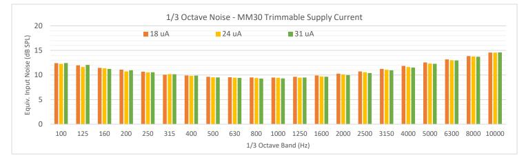
Equivalent input noise is slightly higher with lower supply current; as buffer current is the main factor in the dominant thermal noise in the middle frequency bands. Acoustic noise begins to dominate closer to the acoustic peak frequency.
