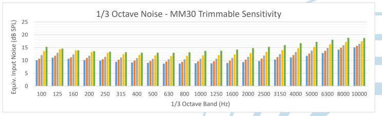
Equivalent input noise increase with decreasing sensitivity is due to the gained-up input-referred electrical noise.
