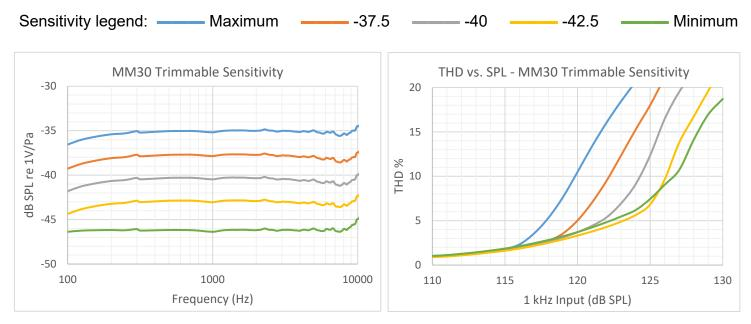
1kHz sensitivity for this data was trimmed via hard-coded maximum and minimum values, plus three precise values within the recommended range. Improved (increased) AOP with decreasing sensitivity is caused by the decrease of the output signal amplitude, and the resulting decrease in the signal clipping that causes distortion.
