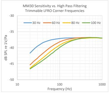
High pass filter trimming targets the frequency point where sensitivity is a certain value relative to 1 kHz sensitivity, commonly known as the corner frequency for low frequency rolloff (LFRO). The trim settings for the data above were for -37.0 dB SPL sensitivity at 1 kHz, and the industry standard -3.0 dB with respect to that for the frequency targets shown in the legend.
