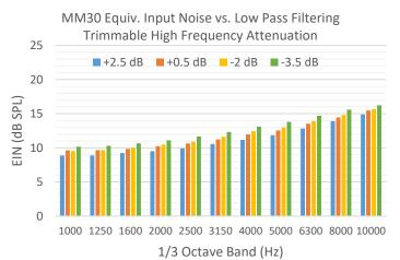
Increasing attenuation via high pass or low pass filtering introduces more thermal noise at the ASIC with the activation of more capacitors and resistors with more aggressive trimming.
