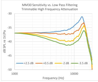
Low pass filter trimming targets the sensitivity at a certain high frequency point, commonly 10 kHz, relative to 1 kHz sensitivity. The trim settings for the data above were for -37.0 dB SPL sensitivity at 1 kHz, and the values shown in the legend for 10 kHz sensitivity with respect to 1 kHz sensitivity.
