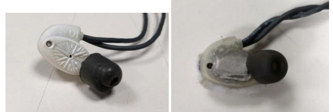
Figure 10 Sheltered mic without and with screen protection. Ribs prevent port from sealing against skin.
