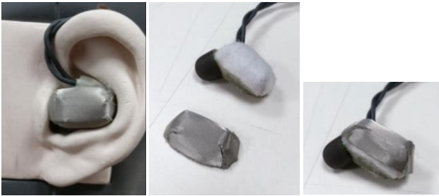
Figure 8 Appearance of streamlined headset. Middle picture shows felt lining over headset body.
