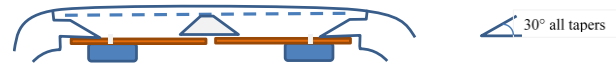
Figure 7 Isolated chambers should be made for each microphone behind the wind screen
