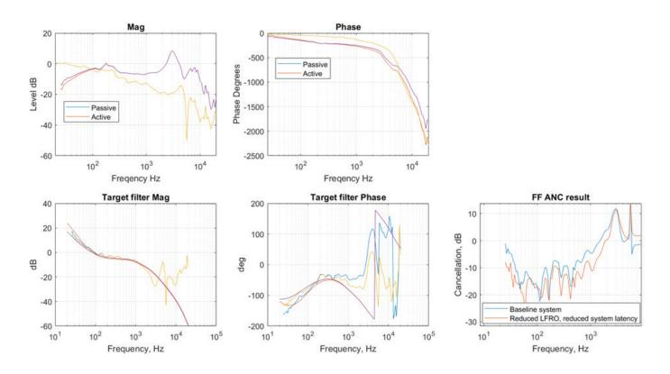
Should it be concluded that FF mic LFRO for TWS ANC headsets should be as low as possible? It will improve ANC but there are other system trade offs that are important to take into account. For example, wind noise mitigation. Having too low mic LFRO makes the system too sensitive to wind noise which is rich in low frequencies.
