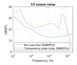
The level of transparency mode hiss drives the requirement to use microphones with as high as possible SNR. Higher SNR and thus lower microphone noise expands the range of use cases for transparency mode where the user will not experience the hiss.
