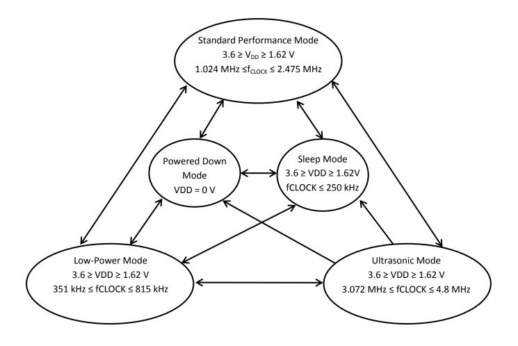
Note: Do not power up into ultrasonic mode. Do not wake-up from sleep mode into ultrasonic mode.
