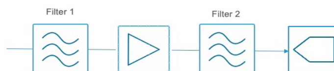
Figure 12. An example of a direct sampling receiver.
